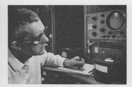
A TRANSFER STANDARD is being used by Harold Beadersted (4632-2) to calibrate a voltmeter.
